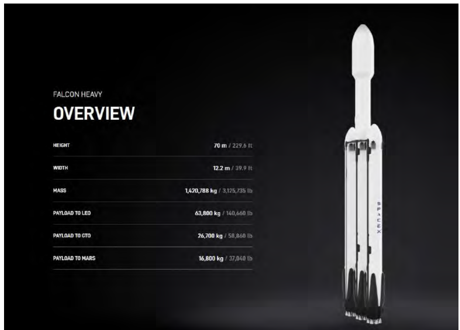
SpaceX Falcon Heavy Rocket, consisting of 3 Falcon 9 rocket cores, is one of the most powerful rockets. Falcon Heavy can lift almost 64 metric tons (141,000 lbs) into orbit. Screenshot: SpaceX
