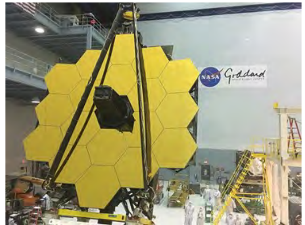
Main mirror assembled at Goddard Space Flight Center, May 2016.
