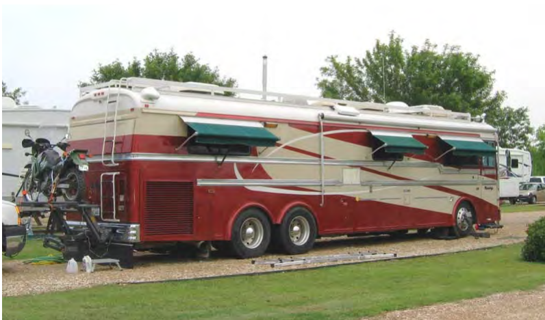
ABOVE: Side view of a very unique installation by Mike Kane, KB1JTB. He had a large piece of diamond plate attached to the roof of his motor home. The antenna, a Scorpion 680, is hinged at the bottom, so once parked, he raises the antenna, and he's in business. Albeit expensive, it sure eliminates the hassles of a tripod, or dipole installation, and is probably as efficient, all considering. Photo courtesy k0bg.com/otrrv.html
