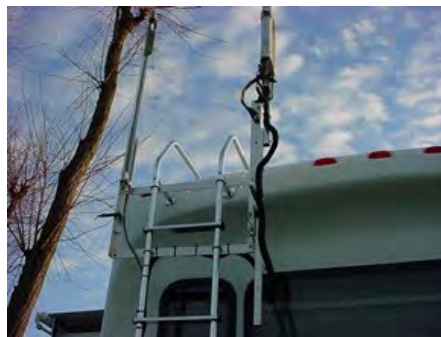
High Sierra HF Screwdriver Antenna with hinged mount attached to ladder. Photo courtesy Bill Moneysmith - W4NFR, from moneysmith.com
