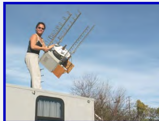
Before a Rover Contest, Carrie Tai-W6TAI hoists an equipment box and antenna system atop a camper. This unit, which includes transverters and amplifiers for four microwave bands as well as antennas for six bands, weighs about 50 pounds, far more than you might suspect from the way she's swinging it around. Photo and caption courtesy of The N6NB Rover Page, overbeck.com/rover
