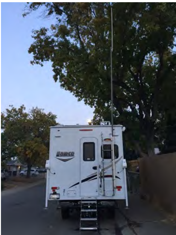
Use your RV's ladder to assist in mounting your antenna. Photo courtesy Paul Young, Pinterest
