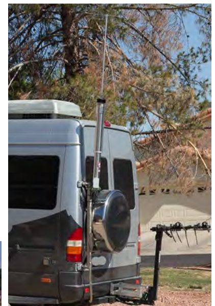
Mark Goldberg's (W7MLG) Great West Sprinter RV with the antenna fully up. The top of the cap hat is still below 13'6", which is a typical minimum clearance for US overpasses. Photo courtesy Mark Goldberg, Peoria, AZ
