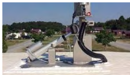
Another HF Screwdriver antenna mounted right on top of an RV. Brian Kress KB3WV decided to fix the hole in his roof by mounting this! Image courtesy Brian Kress
